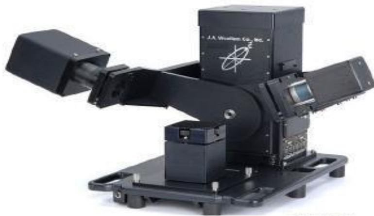
Ellipsometric Spectrometer Lab SIC in Department of Physics
